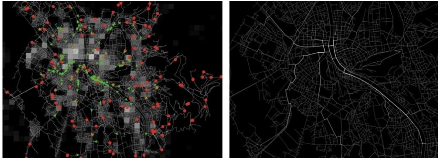
Fig. 5. Agent-based model simulation of bicycle traffic: randomly distributed origin-destination relations with agents (left) and most frequently traversed segments in the network (right). Preliminary results from an ongoing study.
